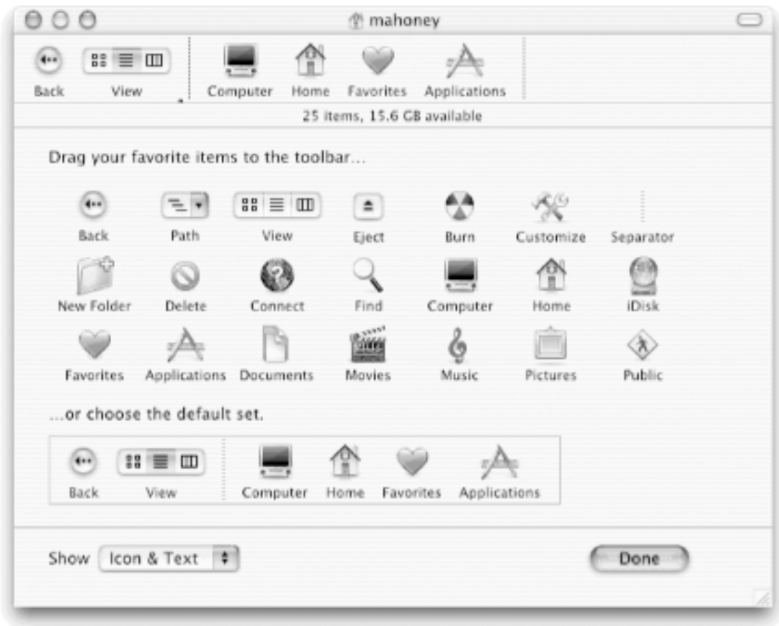
Figure 1-26. For quick access, drag icons from the View pane into the toolbar
