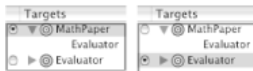
Figure 11-5. Targets pane - adding Evaluator to MathPaper target (left) and selecting Evaluator as active target (right)
